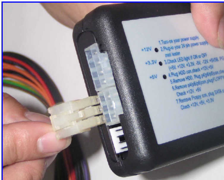
2d) Health Power Check on Hard Drive/CDRom Drive Power Supply Cable:
